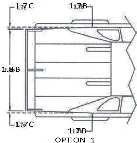
REAR DECKS MUST TAPER FROM SEVENTY-SIX INCHES (76"), AS MEASURED AT THE TOP OVER THE REAR HUBS, UNIFORMLY BACK TO
